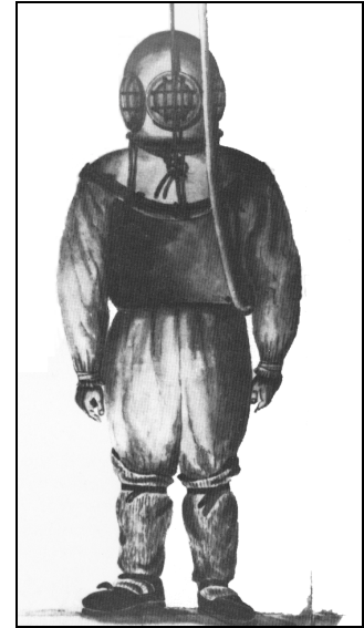
Figure 1-5. Siebe's First Enclosed Diving Dress and Helmet.
